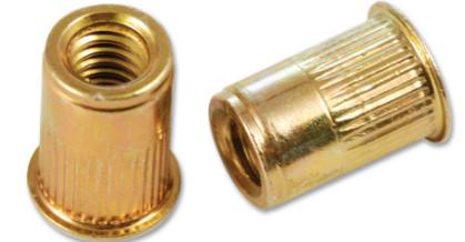
Other MK design benefits include superior thread strength, outstanding corrosion resistance, and prevention of thread dilation due to the increased cross-sectional thickness of the thread area.
